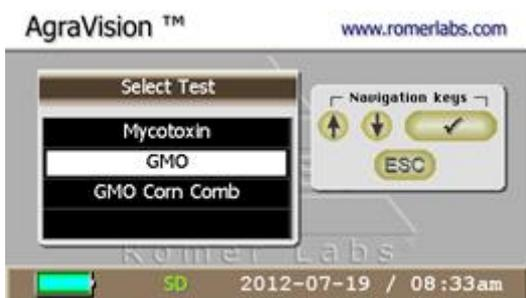
4. By pressing ↑ and ↓ select the strip position that corresponds to the position of the strip inside the tray and press "✓".
