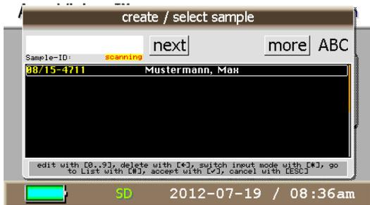
7. Assign the next strip position according to steps 4., 5. and 6. or press the "#" key to skip the next tray position.
